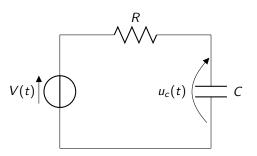
We denote *R* the resistance and *C* the capacity. The considered input is the voltage V(t) of the source, and the output is the voltage  $u_c(t)$  of the capacitor. This electrical system is governed by the following differential equation:
